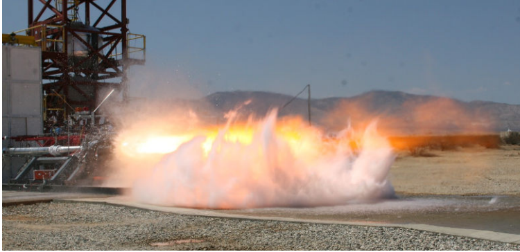
Figure 3: Test firing of the AirLaunch water-cooled LOX/C3H8 VaPak engine at the Mojave Spaceport test facilities.
