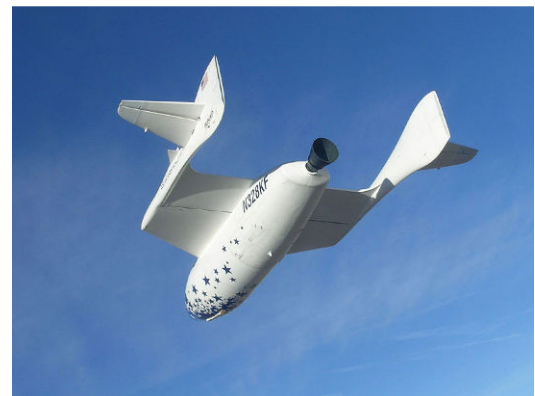
Figure 2: SpaceShipOne used a hybrid rocket engine with VaPak pressurized N 2 O oxidizer.
