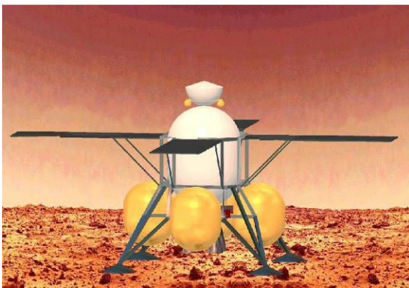
Figure 7: ISRU Mars sample return concept using LOX/Methane propellants. (courtesy of University of Washington)
