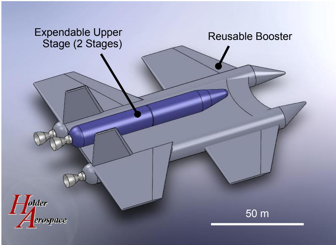
Figure 4: Water takeoff/landing HTHL RLV Booster point-of-departure concept.
