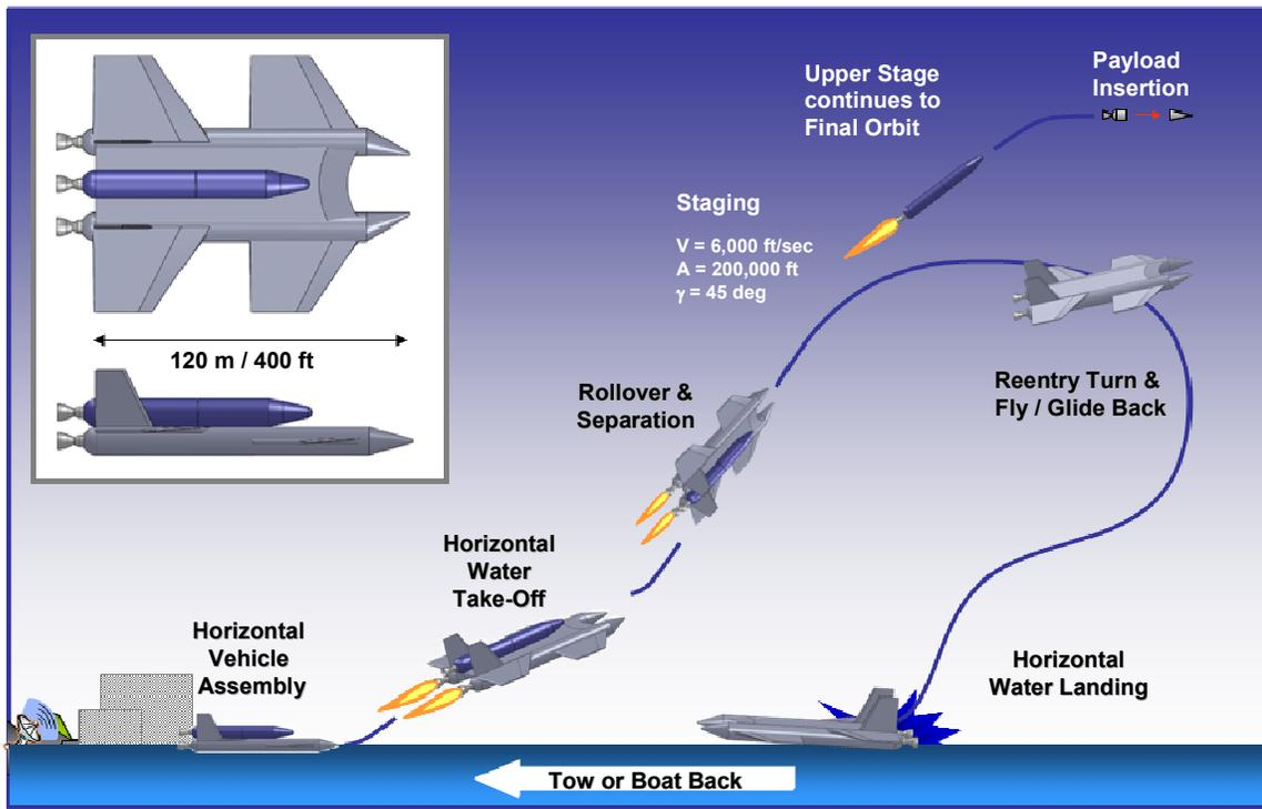
Figure 5: Possible Mission Profile for the water takeoff/landing HTHL RLV Booster concept.
