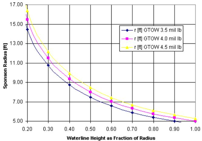
Figure 6: Water-line height vs. tank radius.
